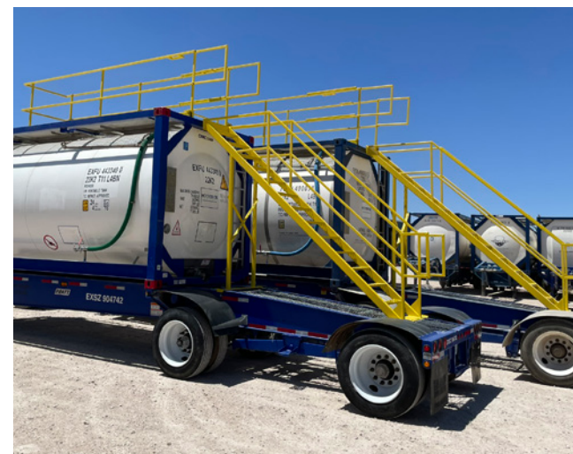
Stairway Mod Installed on 24,000 Liter ISO
