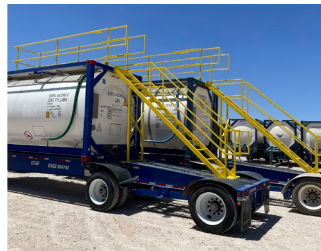
Stairway Upgrade Installed on 24,000 Liter ISO
